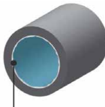
A protective layer of Orthophosphate forms to prevent pipe from corroding.
